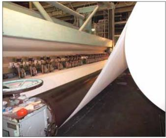
The slitter rewinder can produce various sized rolls at diameters up to 68-in., with width dependent basically on the size of the truck.
