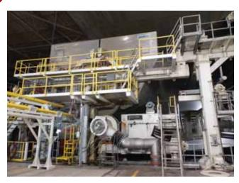
The 12-ft.-dia. PMT yankee dryer, a grooved cast Iron unit with six condensate headers, was shipped from Europe, unloaded at Norfolk, Va., and delivered by truck to the mill.
