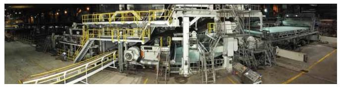
Wide-angle view of PM 6, with the fourdrinier forming section on the right, yankee dyer and hood in the center, and after-dryer section on the left.
