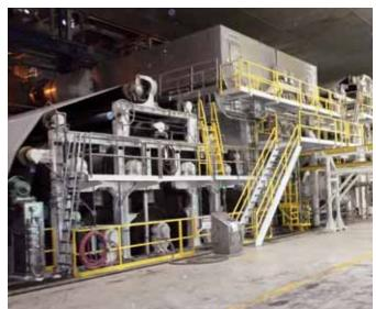
The after-dryer section is comprised of eight dryer drums from the existing fine paper dryer section that were reconfigured and set up to handle tissue.
